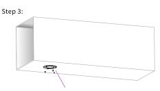
Lock the mounting plate to the ventilation duct with screws.
