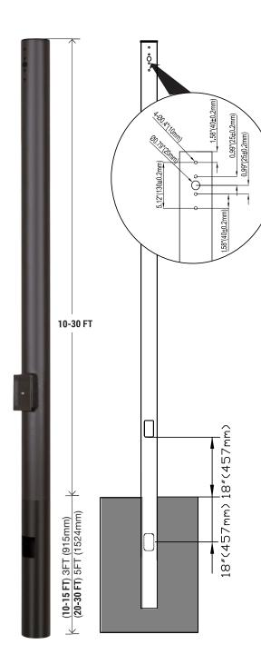
The WSD LED INC Series Direct Burial Straight Round poles are built from high strength steel tube and are available side drilled for arm mounted area lighting luminaires or with tenon mounts for flood and post top luminaires. Typical area lighting applications include retail centers, industrial parks, schools and universities, public transit and airports, office buildings and medical facilities. Mounting heights of 10 to 30 feet can be used based on selected luminaire application.
