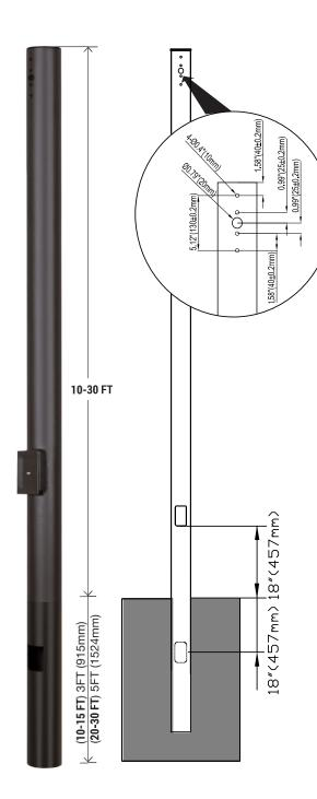
The WSD LED INC Series Direct Burial Straight Round poles are built from high strength steel tube and are available side drilled for arm mounted area lighting luminaires or with tenon mounts for flood and post top luminaires. Typical area lighting applications include retail centers, industrial parks, schools and universities, public transit and airports, office buildings and medical facilities. Mounting heights of 10 to 30 feet can be used based on selected luminaire application.
