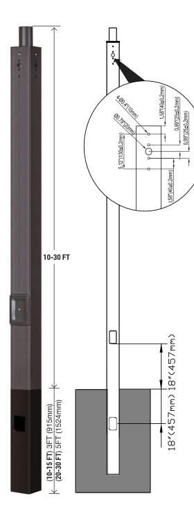
The WSD LED INC Series Direct Burial Straight Square Steel poles are built from high strength steel tube and are available side drilled for arm mounted area lighting luminaires or with tenon mounts for flood and post top luminaires. Typical area lighting applications include retail centers, industrial parks, schools and universities, public transit and airports, office buildings and medical facilities. Mounting heights of 10 to 30 feet can be used based on selected luminaire application.
