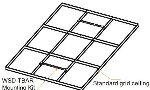
WSD-TBAR Mounting Kit for Emergency LED Driver When emergency led drivers can not be installed on the LED lights such as LED downlights, LED panel lights&LED troffer. We can install the emergency led drivers on the WSD-TBARs and WSD-TBARs are installed on the grid ceiling.
