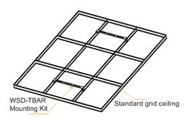
WSD-TBAR Mounting Kit for Emergency LED Driver When emergency led drivers can not be installed on the LED lights such as LED downlights, LED panel lights&LED troffer. We can install the emergency led drivers on the WSD-TBARs and WSD-TBARs are installed on the grid ceiling.
