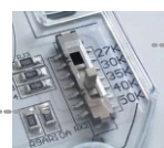
CCT SWITCH 4000K (FACTORY SETTINGS)
