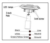
1) Connect the AC wire of the lamp as shown in the picture, then insert the lamp into the 3-Inch pole.
