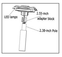
3) When the light pole is 2.38 inches, a 2.5 inch adapter shall be installed on the fixture.
