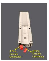
Female 3 pin JST SM Connector to light up the joiners.
