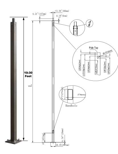
The WSD LED INC Series Square aluminum poles are built from high strength aluminum Square tube and are available side drilled for arm mounted area lighting luminaires or with tenon mounts for flood and post top luminaires. Typical area lighting applications include retail centers, industrial parks, schools and universities, public transit and airports, office buildings and medical facilities. Mounting heights of 10 to 30 feet can be used based on selected luminaire application.
