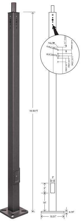
The WSD LED INC Series Straight Square Steel poles are built from high strength steel tube and are available side drilled for arm mounted area lighting luminaires or with tenon mounts for flood and post top luminaires. Typical area lighting applications include retail centers, industrial parks, schools and universities, public transit and airports, office buildings and medical facilities. Mounting heights of 10 to 30 feet can be used based on selected luminaire application.
