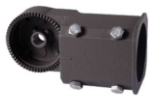
WSD-NEWSBSF2-D Slipfitter Mount An optional cast aluminum mast arm adapter secures fixture head to nominal 2"(2-3/8"O.D. pipe size) horizontal steel tenon arm.
