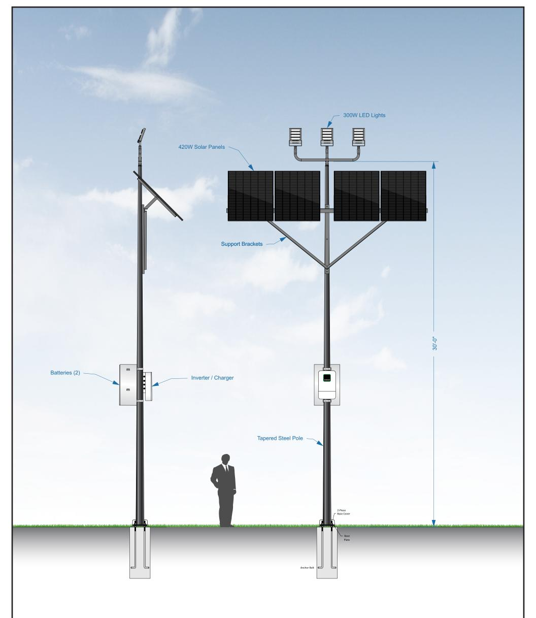
3x300W LED lights with 4x420W solar panels. 2x100 AH / 25.6V batteries. Tapered steel pole with steel angle support brackets and bullhorn mounting arms for lights, steel angle braces for solar panels. Concrete footings (footing dimension determined by registered engineer). Lithium batteries mounted in weather tight enclosures. Discharge = 5.5 hours at 100% full power.
